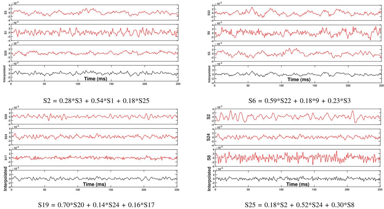
Fig. 7. First three plots in all sub-figures show the actual acceleration patterns for the real texture models, whereas the last plot shows the weighted synthesized acceleration pattern at the location of the new virtual texture. The authored signal is synthesized by adding the three original signals according to the weights given in the equation below each sub-figure.
