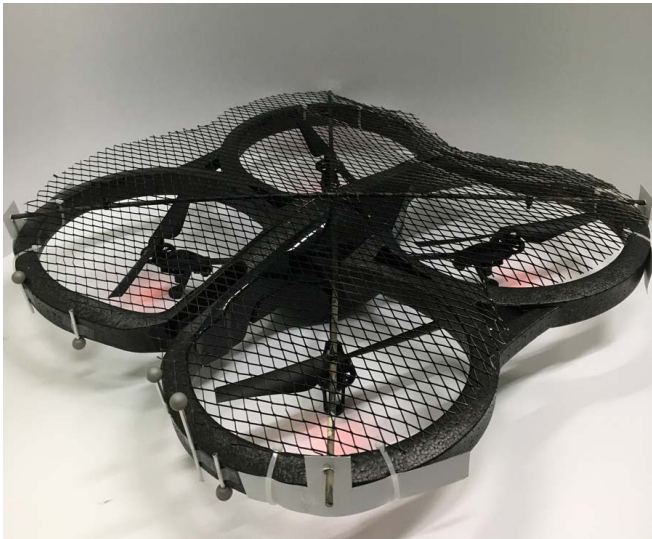
Fig. 1. The final design of the HapticDrone with the safety cover and tracking markers in place.
