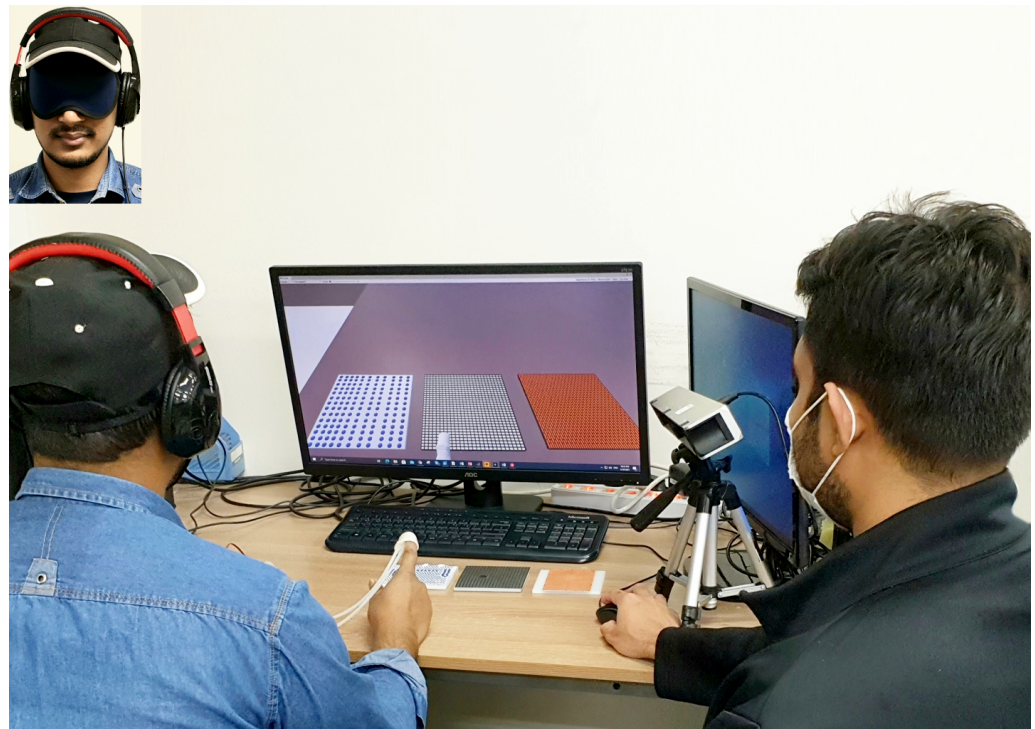
Figure 10. Similarity experiment. The participant compares a real–virtual pair of objects. The operator sitting to the right of the participant replaces the real and virtual samples and records the reported similarity ratings.
