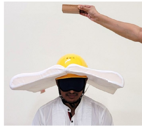
Fig. 12 Perceptual experiment. The participant compares the virtually rendered impact feedback and feedback from real objects falling. A safe guard was attached to the outside part of the helmet for safety reasons
