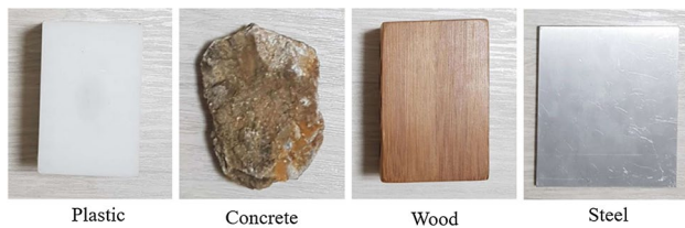
Fig. 7 Four objects: Plastic frame, Concrete type broken brick, Wood type broken beam, and Steel type ceiling part used for the experiments
