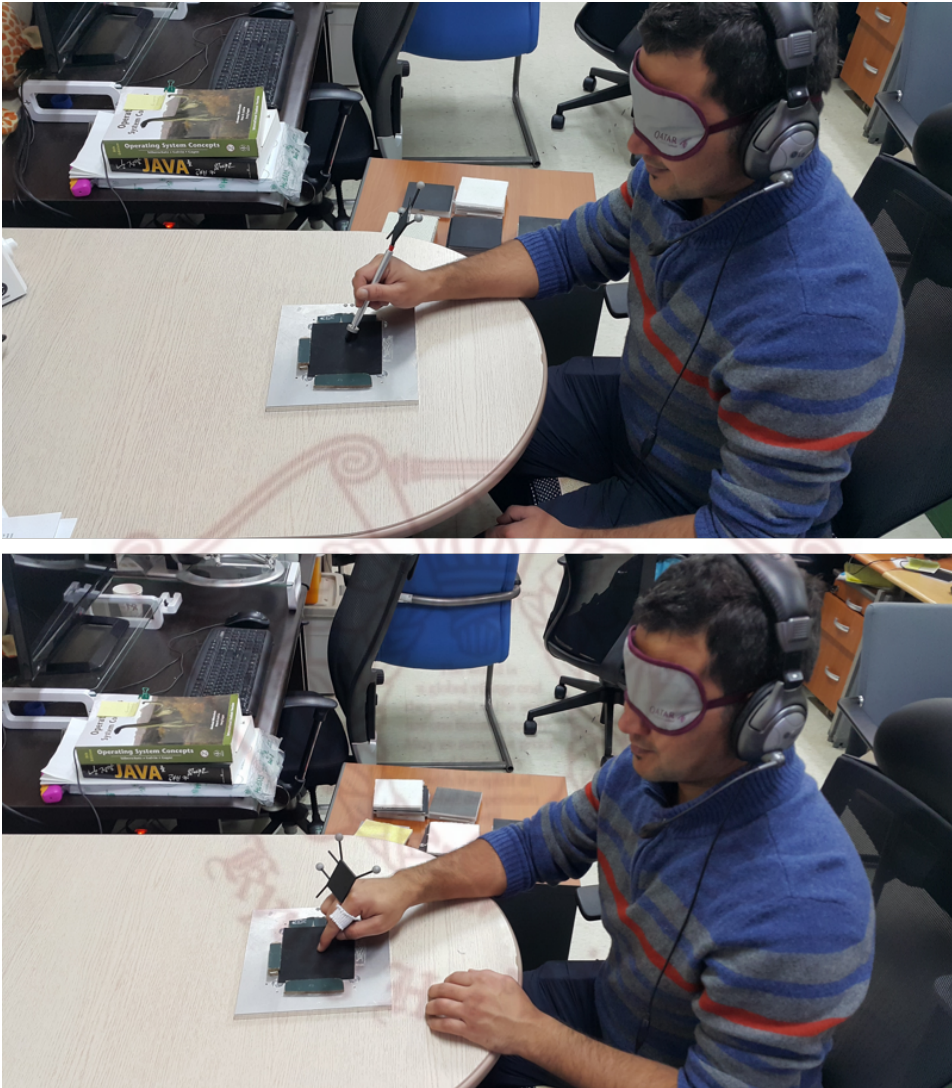
Figure 8.2: The experimental setup and environment for the experiment. Top is tool based interaction, bottom is bare handed interaction.
