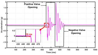
FIGURE 12. System's response time measurement result.
