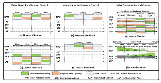
FIGURE 6. Valve control mechanism to produce different modes of actuation.
