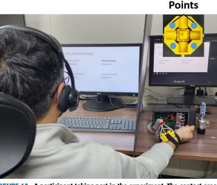
**FIGURE 13.** A participant taking part in the experiment. The contact area is also highlighted creating no contact force between the body site and the end-effector when attached to the body.
