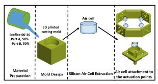
FIGURE 4. Fabrication procedure of the air cell.
