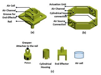
**FIGURE 3.** (a) Normal Actuation Unit (NAU), (b) Lateral Actuation Unit (LAU), (c) Components used to form the complete actuator.
