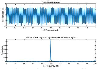
**FIGURE 9.** Time domain and respective frequency spectrum of the 100 Hz signal rendered at 7.5 psi.
