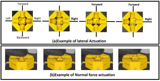
FIGURE 2. (a)Example of actuation in 2D area. The first picture on the left shows the actuator in its default state of no actuation, the second picture shows lateral motion to the right, the third picture shows actuation forward, and the rightmost picture shows right-forward actuation. (b) Example of actuation in the normal direction. The pictures from left to right show increasing normal force as the end-effector moves up.
