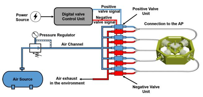
FIGURE 5. Pneumatic actuation control system.
