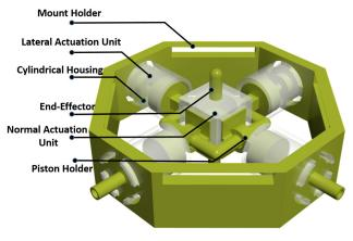
FIGURE 1. 3D Design of Pneumatically controlled Multi-Modal Tactile Actuator (MMTA).
