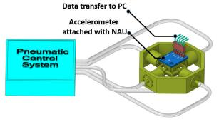
FIGURE 7. Acceleration measurement setup.
