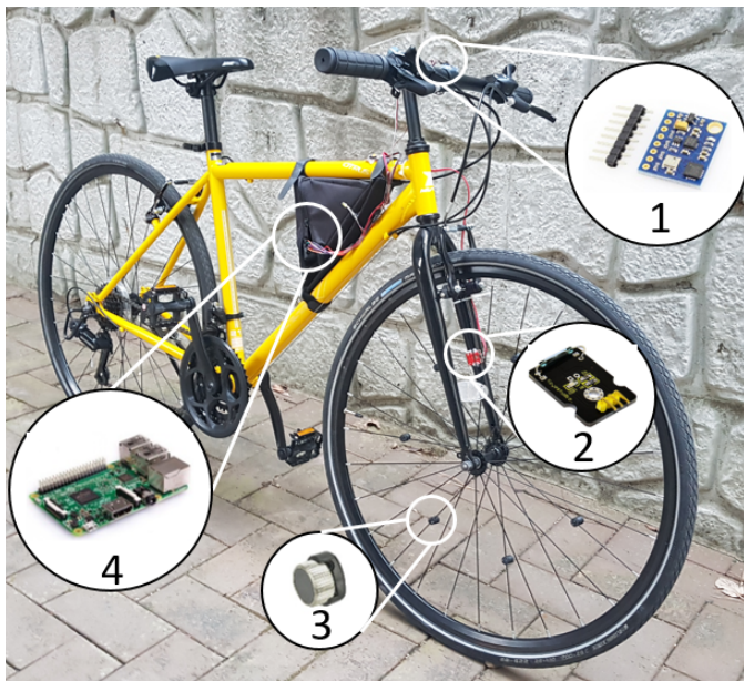
Fig. 1. Data Collection Bicycle: 1) ADXL 345 digital accelerometer; 2) Hall sensor; 3) Magnets; 4) Raspberry Pi.
