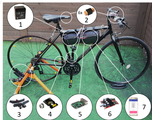
Fig. 4. Rendering System: 1) Power Supply; 2) Six Haptuators; 3) Magnetic Resistance Unit; 4) Hall sensor and Magnets; 5) Raspberry Pi; 6) Amplifier; 7) Samsung Galaxy S7
